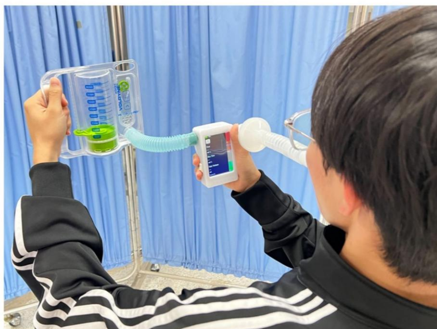
Figure 2. Validation setup of the Breathive device and the Voldyne device.
