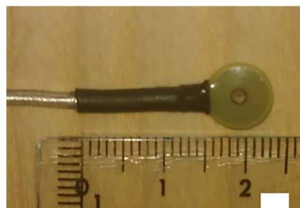
Figure 3. Head Position Indicator (HPI) coil used for co-registration purposes. Reprinted from [31]. (Copyright 2018 PLOS) Image reproduced as per terms of CC BY 4.0 license.
