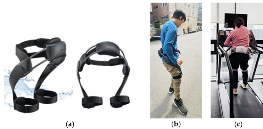
Figure 1. Powered wearable exoskeleton and gait training setup. (a) Front and rear views of the Samsung Bot Fit powered lower-limb exoskeleton. (b) Lateral view of the participant wearing the exoskeleton during overground gait training. (c) Posterior view of a different individual demonstrating treadmill-based use of the exoskeleton, shown for illustrative reference only and not depicting the study participant. Panel (b) is a photograph of the actual study participant, taken with written informed consent. Panel (c) shows a different individual and is included solely to illustrate device positioning during treadmill-based training.
