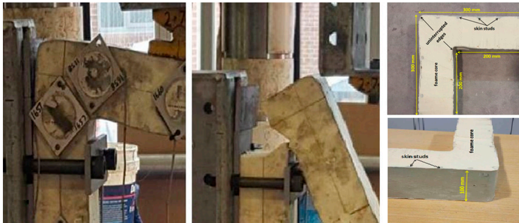
Figure 10. The ultimate deflection and the mechanism of collapse and dimensions of the connection.
