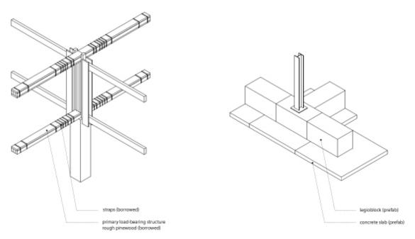
Figure 6. Different building details that were designed for de-/reconstruction.
