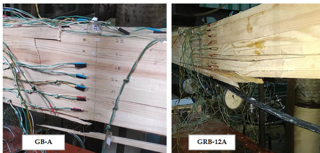
Figure 8. Fracture pattern of GB-A and GRB-12A beams.
