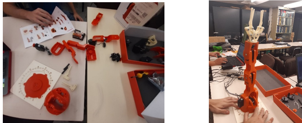
Figure 8. Braccio. Arduino-based robotic arm.
