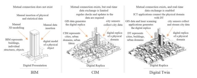
Figure 5. Applications of digitalisation in the built environment: BIM, CIM and DT. Source: Authors.
