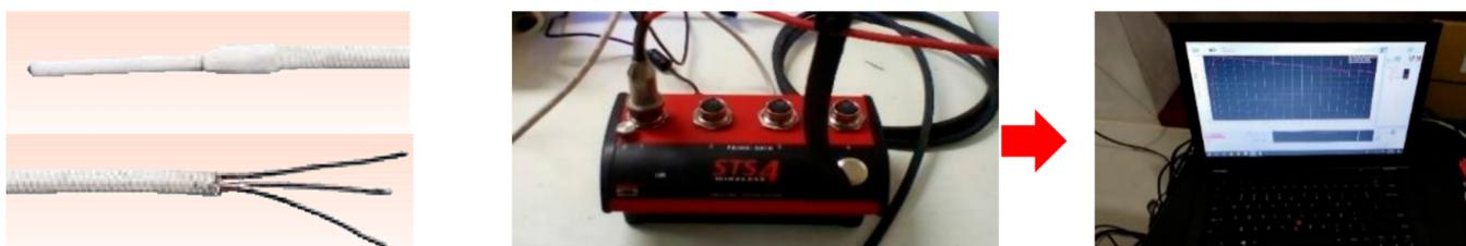
**Figure 4.** High precision thermal RTD sensor (RTD-1PT100K2515-36-T) and data acquisition system.
