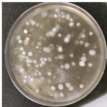
Figure A1. Example of a Petri dish with MEA medium after incubation, sample made with a 6-stage Andersen impactor.
