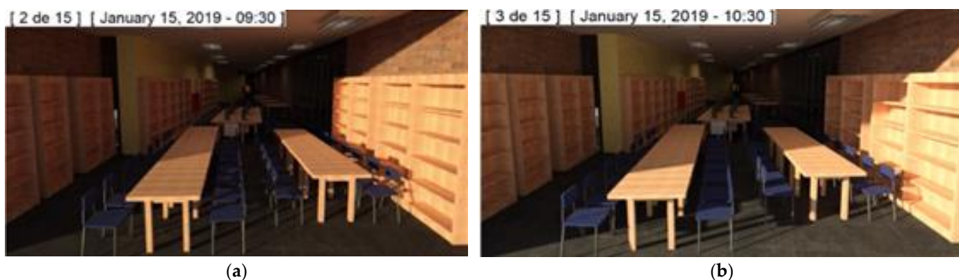
Figure 7. Two frames from one of the daylight simulation videos, showing the evolution of the sun's rays inside the library's study room through the 15th of January.
