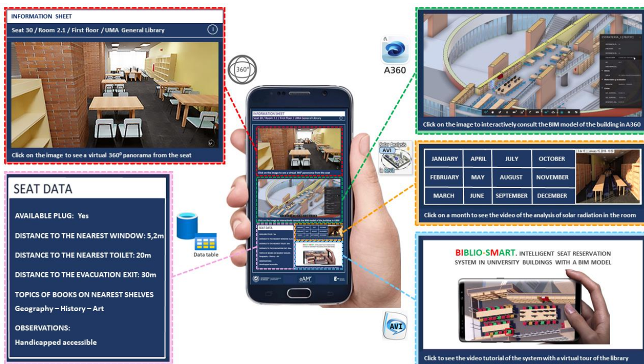
Figure 10. Biblio-Smart app interface designed to consult information of interest for the reservation from BIM model data, with its expanded options and icons of the file format or tool used.
