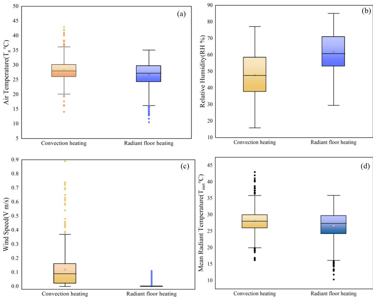
**Figure 4.** Indoor thermal parameter distribution: (a) air temperature, (b) relative humidity, (c) air velocity, and (d) mean radiant temperature.
