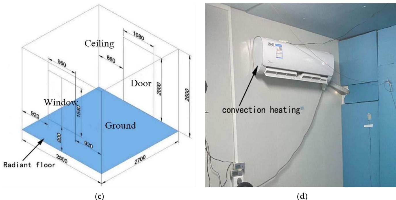
**Figure 1.** (a) Climate chamber schematic diagram. (b) Shaded window in the climate room. (c) Radiant floor heating and (d) convection heating for wall-mounted air conditioners.
