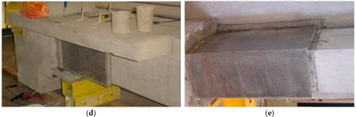
**Figure 4.** Execution of the UFRG jacketing. (a) Casting of the reinforced concrete beam; (b) Concrete surface prepared with water and sandblasting, and casting holes; (c) Application of the unidirectional and non-woven steel fibre mat; (d) Formwork setting for gravity casting with external vibration; (e) Specimen final aspect.
