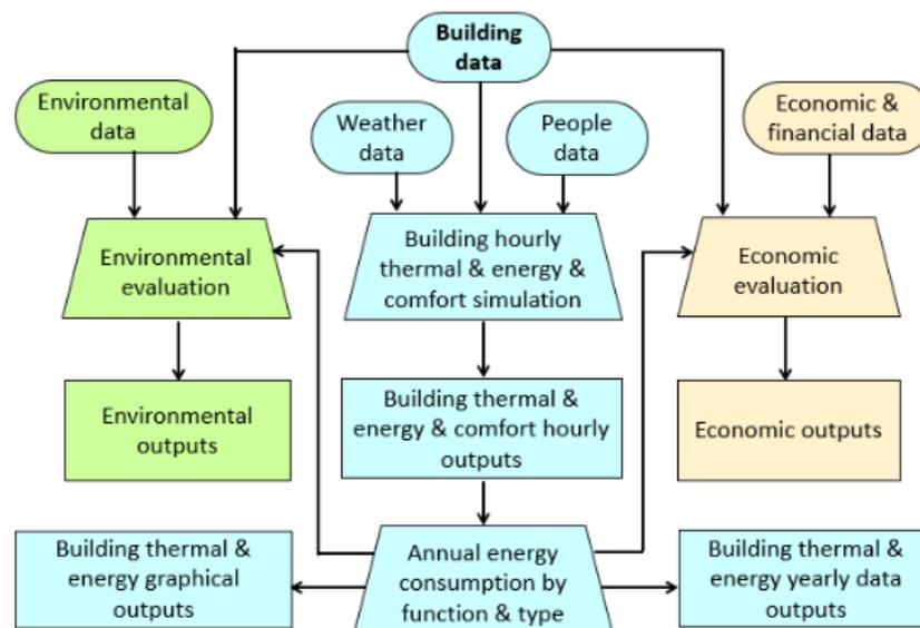
**Figure 1.** Global block diagram of the SEnergyEd calculation methodology.
