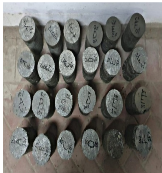
Figure 5. Final cylindrical blocks made of SPFRP.
