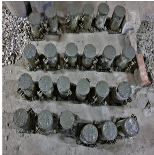
Figure 6. Construction of the samples in the cylindrical molds.
