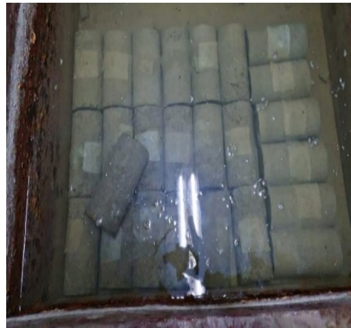
Figure 7. The samples under the curing process to obtain wettability.
