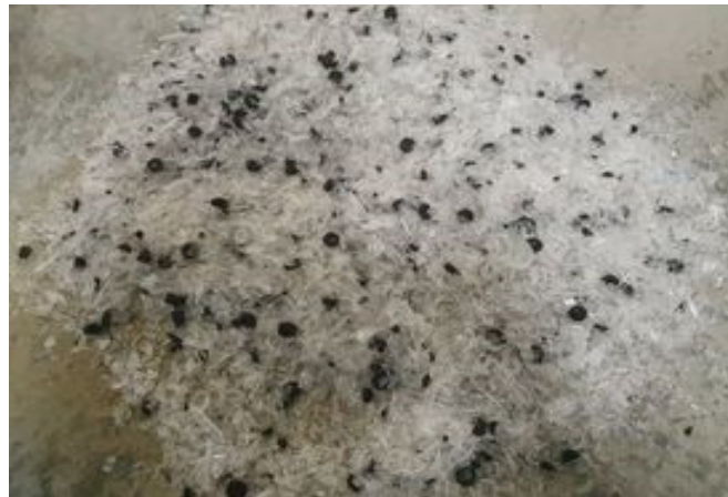
Figure 4. Crushed syringe polypropylene plastic particles.
