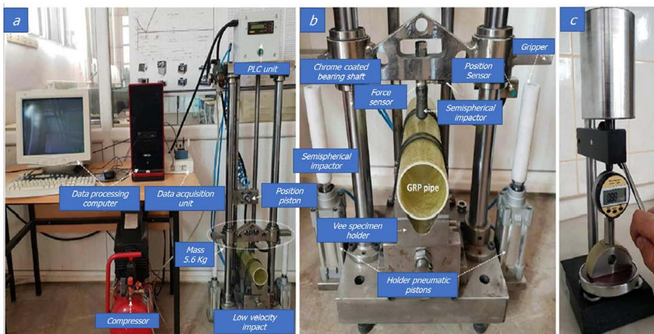
Figure 2. (a) Low-velocity impact test stand and data logging system, (b) anti-rebound system, and (c) shore D hardness tester [37,38].
