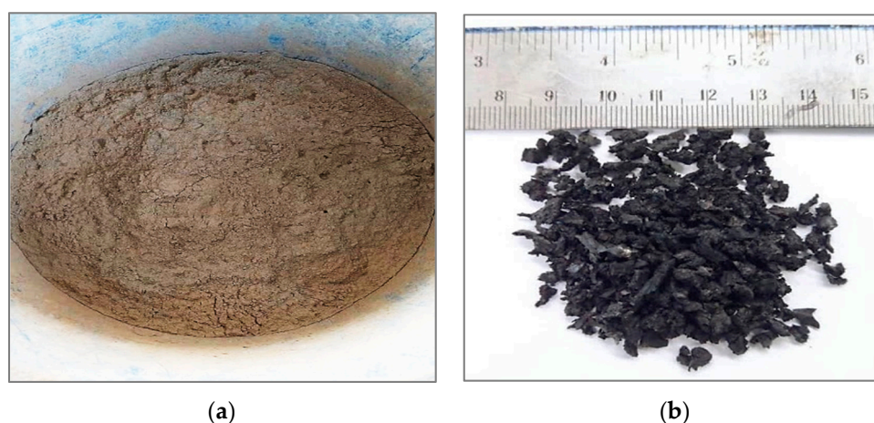
Figure 1. Some of the key ingredients (a) Class F fly ash; (b) crumb rubber.
