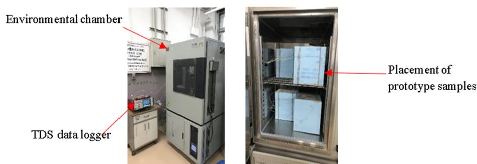
**Figure 2.** Environmental chamber for heat cycle test.
