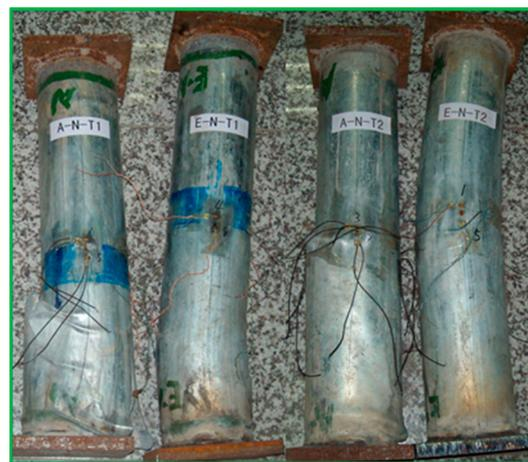
Figure 3. The columns' failure modes.
