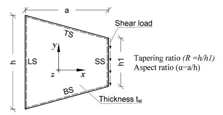
Figure 2. Parameters and schematic drawing for pure shear loading models.
