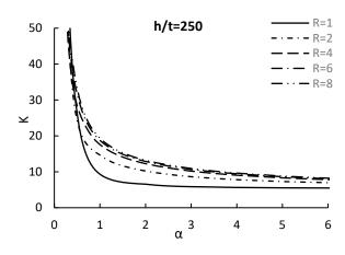
**Figure A1.** Shear buckling coefficient k vs. normalized length  $\alpha$  for different slenderness ratios.
