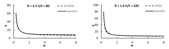
Figure 11. Verification of the proposed formula with new cases not included in the best fit process.
