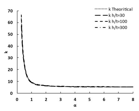
Figure 4. Theoretical and FEM buckling coefficient for rectangular web plates.
