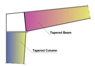
Figure 1. Steel tapered sections in frame structure.
