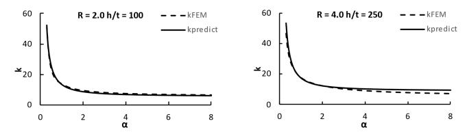
Figure 9. FEM and predicted buckling coefficient.
