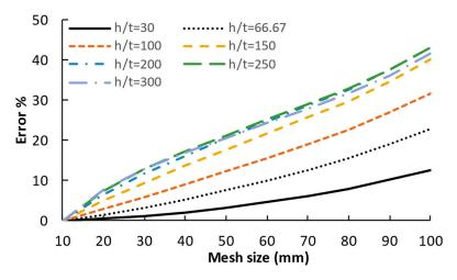
Figure 3. Convergence analysis of FEM and accuracy results.
