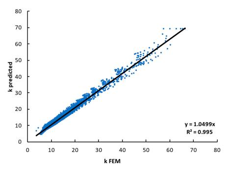
Figure 10. Verification of the predicted buckling coefficient of prismatic web plate of shear load.
