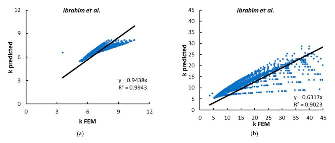
**Figure 13.** Performance of Ibrahim et al. [26] models: (a) for *R* between 1–5 and  $\alpha$  between 3–8, and (b) for *R* between 1–5 and  $\alpha$  between 0.3–8.
