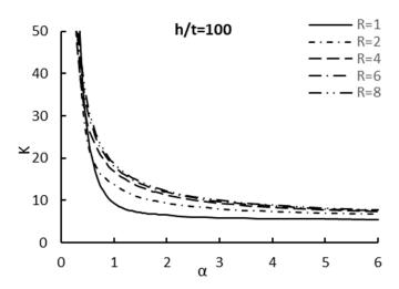
**Figure 5.** Shear buckling coefficient k vs. aspect ratio  $\alpha$  for slenderness ratio equals to 100.
