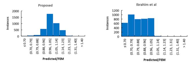
**Figure 14.** Prediction/FEM distribution histogram for *R* between 1–5 and  $\alpha$  between 0.3–8 [26].
