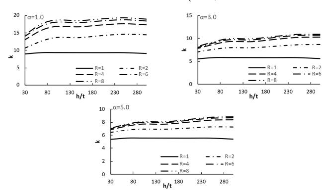
**Figure 8.** Shear buckling coefficient (k) vs. slenderness ratio ( $h/t_w$ ) for several tapering ratios (R).
