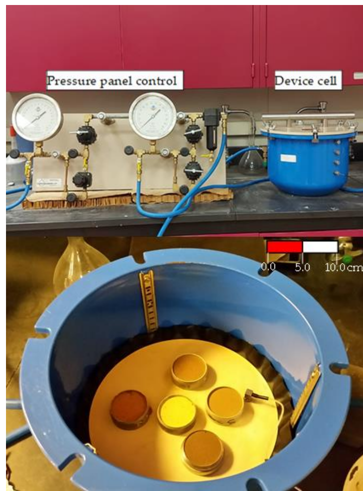
Figure 4. Soil specimen inside pressure plate cell (axis translation technique).
