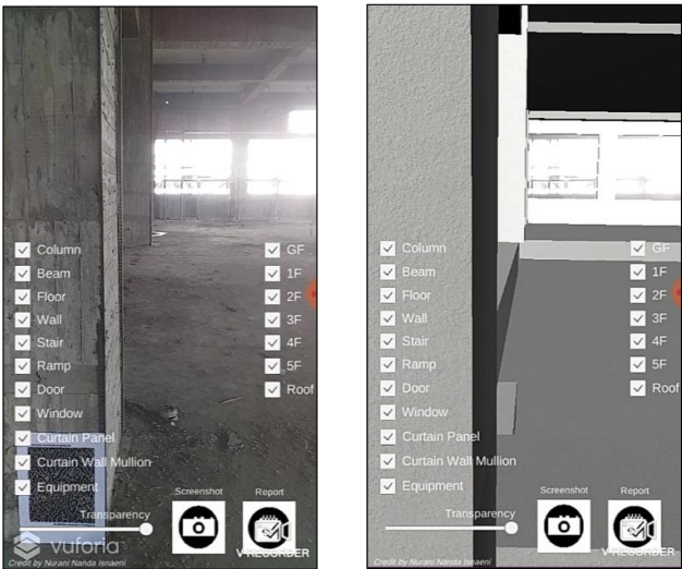
Figure 13. AR-BIM App Prototype Extended Tracking Failure.
