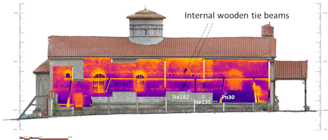
Figure 11. IR thermographs overlaid on the orthophoto of the north façade. Two parallel internal wooden tie beams are discerned, behind the exterior stone layer.
