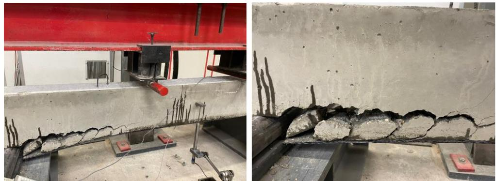
**Figure 9.** Failure modes of strengthened beams.
