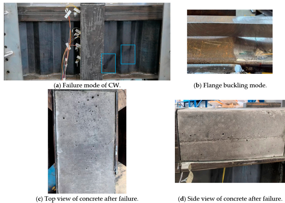
Figure 14. Failure modes of SP-180-2-30.
