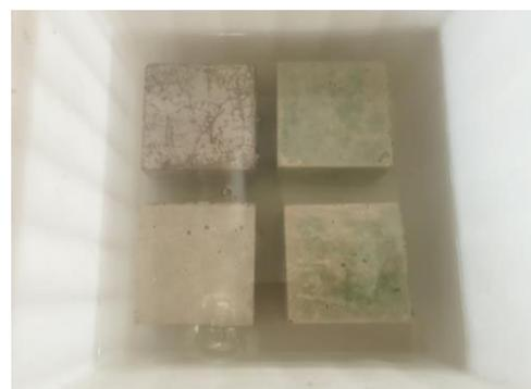
**Figure 4.** Specimen fully soaked.
