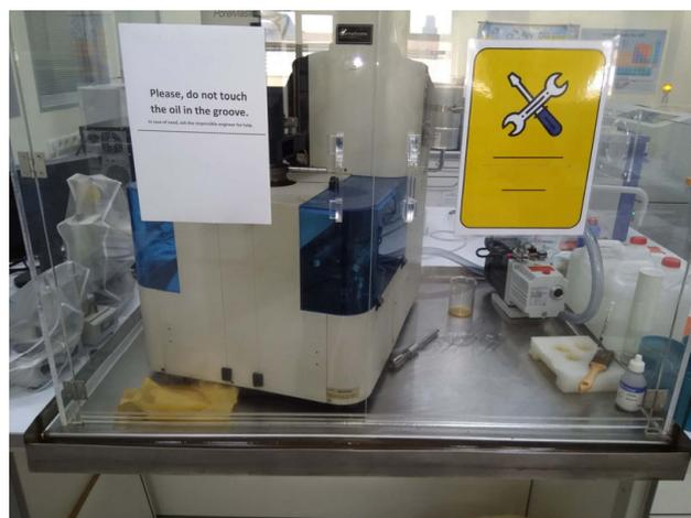
**Figure 14.** American Quanta Pore Master 60 GT mercury porosimeter.
