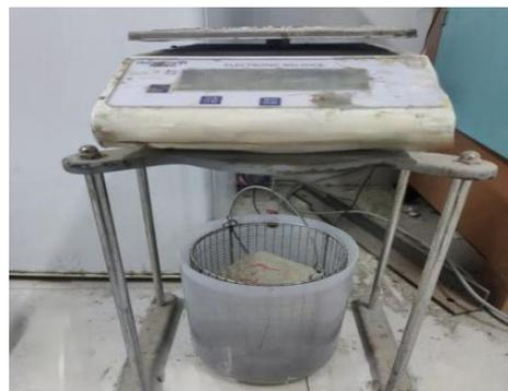
**Figure 6.** Hydrostatical balance.
