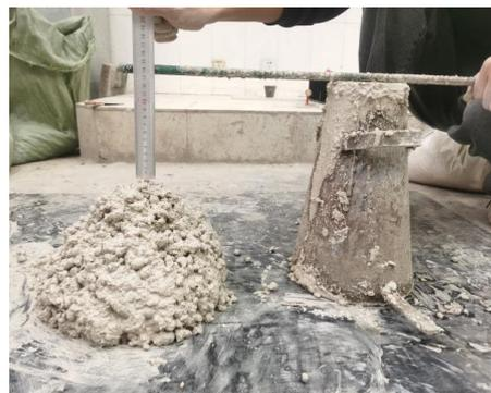
**Figure 3.** Slump of different shell fine aggregate replacement rates.
