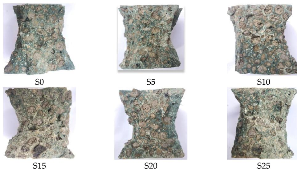
**Figure 12.** Failure interface of the specimen under Compression.
