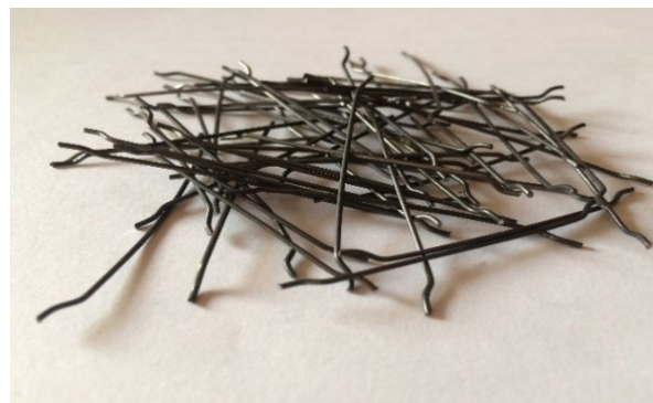
Figure 1. Hooked-end steel fibers.
