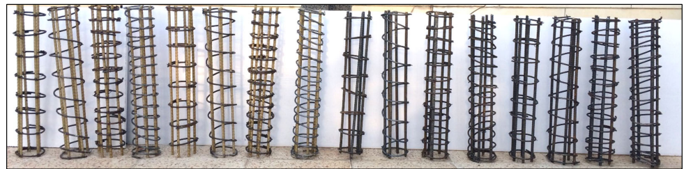
Figure 4. Reinforcement layouts investigated in this study.
