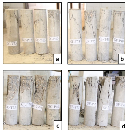
Figure 7. Axially loaded columns after testing with their failure modes: (a) GRCC columns, (b) GRFC columns, (c) SRCC columns, and (d) SRFC columns.
