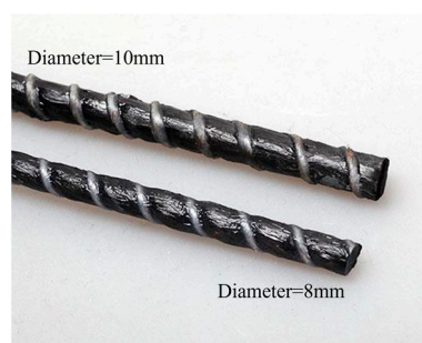
Figure 1. The BFRP used in the test.
