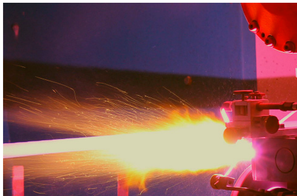
Figure 9. Application of plasma-sprayed Al 2 O 3 coating on the surface of a plain steel bar with a WSP-H 500 torch.
