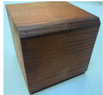
(a) Crack formation during heating (b) color change after heating
