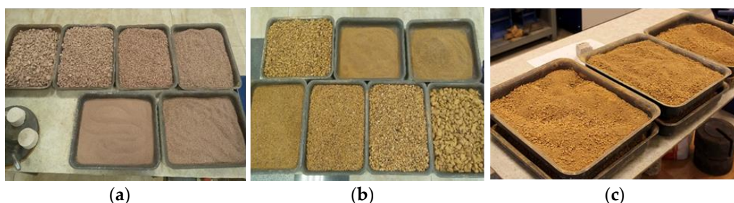
Figure 1. Characteristic images of used tuff sands: (a) Artik, (b) Ani, and (c) Agarak mines.
