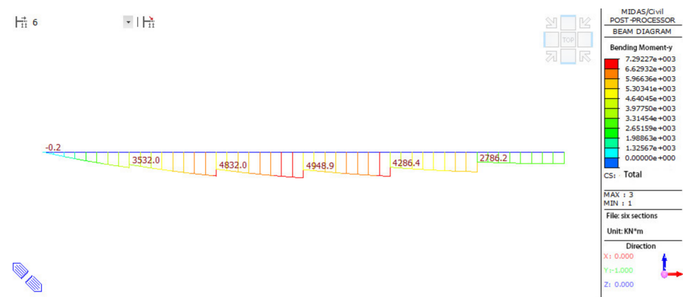
Figure 5. Maximum cantilever state bending moment diagram (unit: kN·m).
