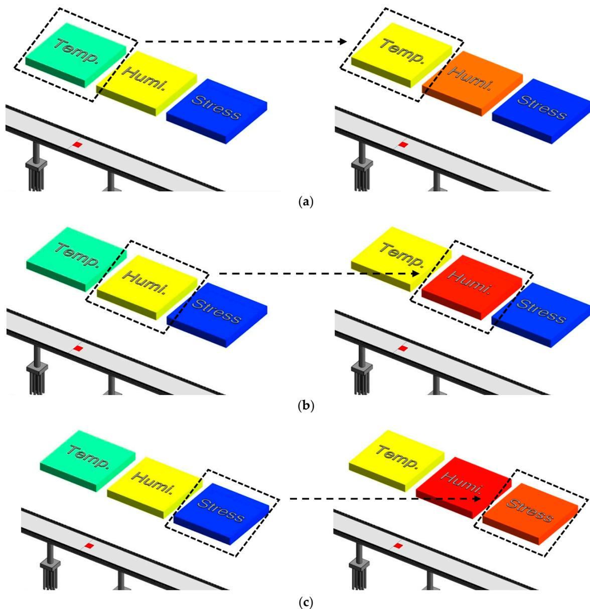
**Figure 8.** Visualization results through Dynamo scripts: (a) temperature, (b) humidity, and (c) stress.
