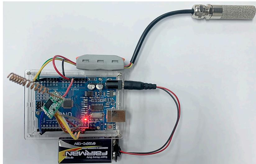
**Figure 3.** Circuit connection between the SHT-31 and Arduino Uno.
