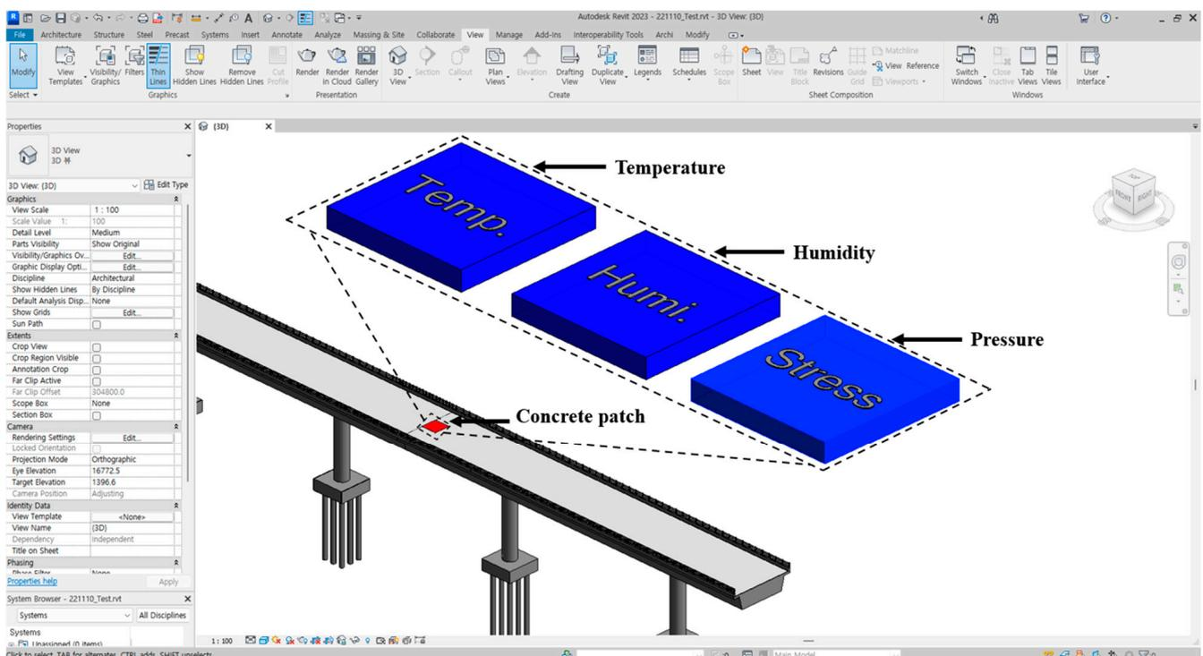
**Figure 6.** A 3D model of the concrete repair area.
