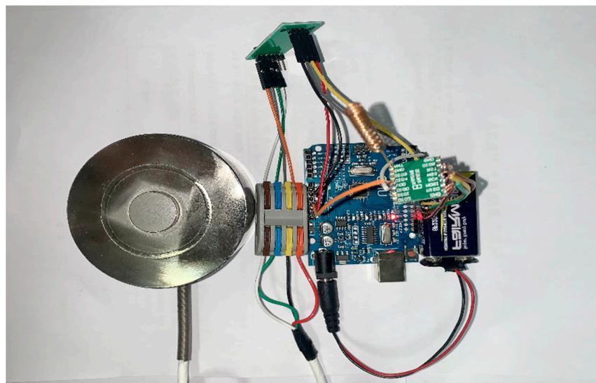
**Figure 4.** Circuit connection between Model 53, HX711 module, and Arduino Uno.
