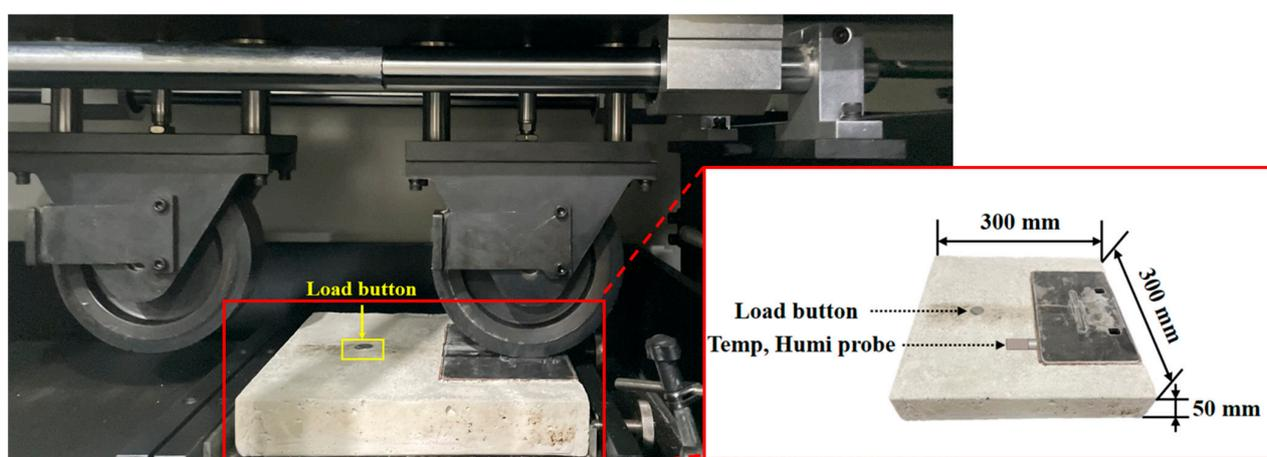
Figure 7. Wheel tracking test for monitoring system verification.
