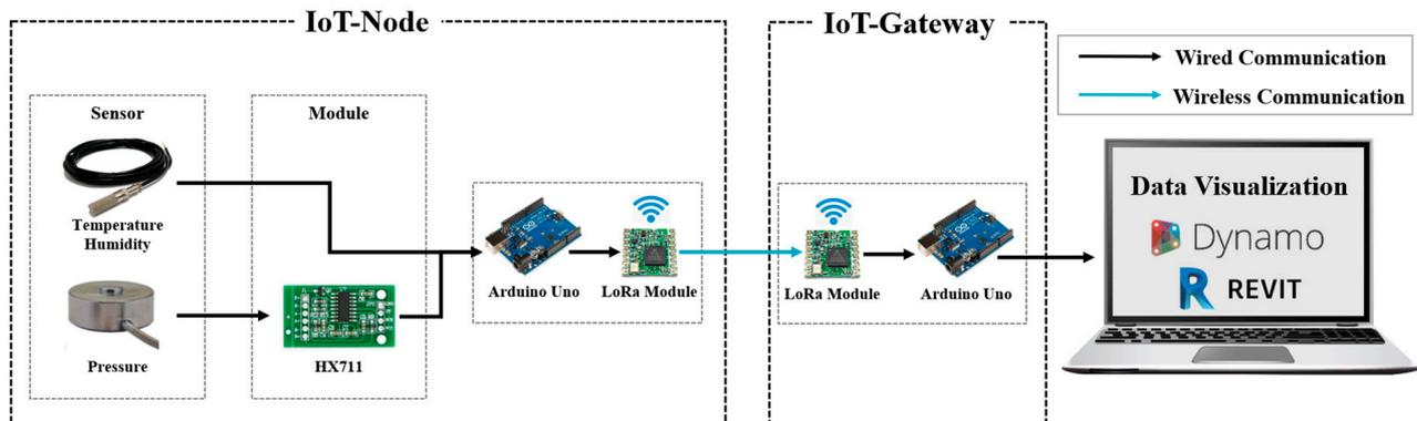
**Figure 2.** The design of the IoT hardware.
