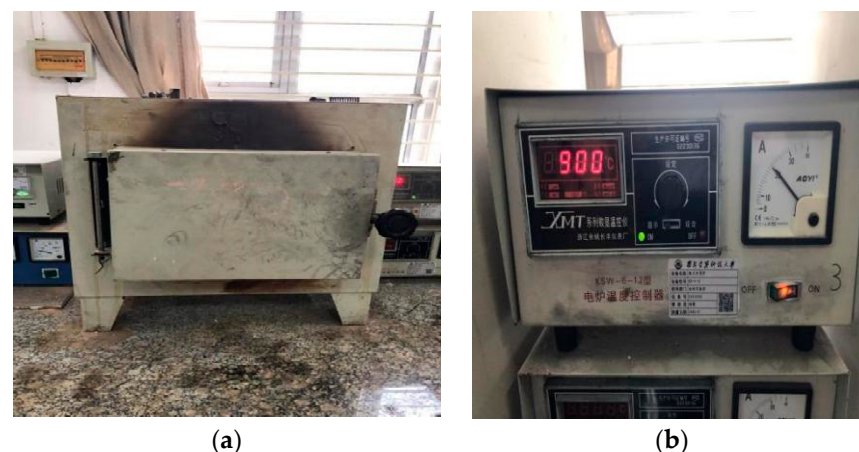
Figure 2. High-temperature test setup [4]. (a) High-temperature electric furnace. (b) Electric furnace temperature controller.
