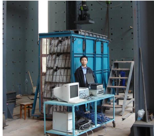
Figure 1. A photograph of the model test of geogrid reinforced soil wall.
