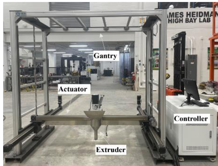
Figure 4. Apparatus of the extrusion-based screw-type 3D printer.
