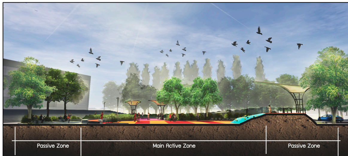
Figure 8. East-West section of the site, representing characterization of active and passive zones and, in blue, “the mountain” device. Credit: the Author.
