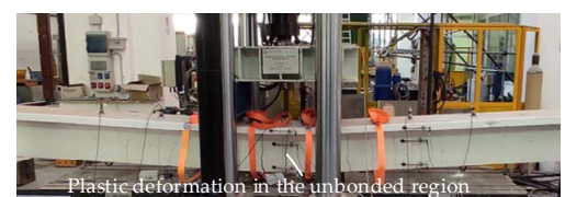
(c) Failure of partially bonded members
