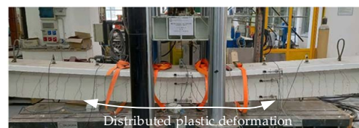
(b) Failure of bonded members
