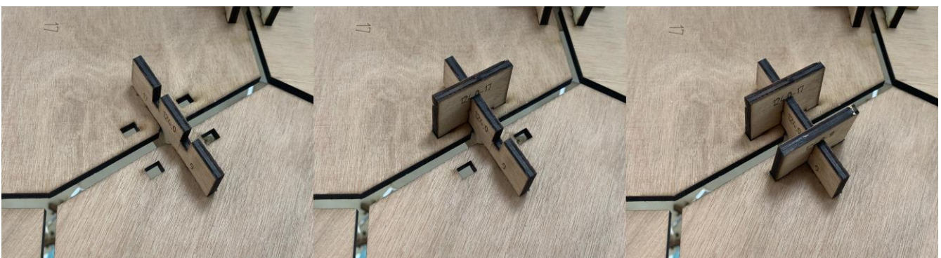
Figure 6. The main connector alone. The Figure shows the main connector and one of the locks. The main connector with both locks corresponds to one edge of the plates.
