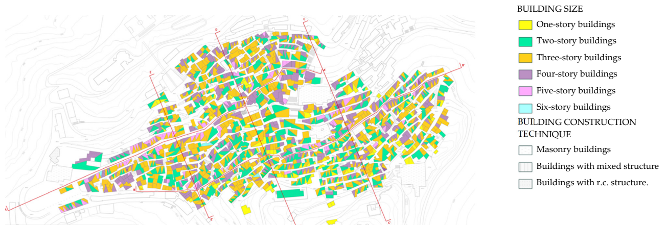
Figure 1. Building stock size and construction techniques (Image prepared by Arch. P. Di Bella).
