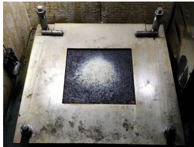
Figure 3. The sample fixing device.
