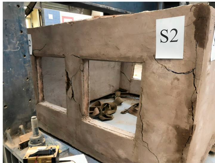
Figure 17. Cracks initiated during testing the infilled specimen.
