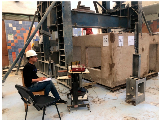
Figure 7. Specimen S2 (the infilled specimen) during testing The scaled structure was tested in the lateral direction in the manner shown in Figures 6a and 8 in the Reinforced Concrete Institute in Housing and Building Research Center (HBRC). The load was applied using an actuator performing a pushover test by a load cell with a capacity of 25 metric tons and a precision of 1%. Horizontal deflections were measured using three linear variable differential transformers (LVDTs) with a 0.01 mm precision. Two LVDTs were assembled in the direction parallel to the load; the third was placed in the perpendicular direction to account for any lateral deflection due to twisting effect as shown in Figures 6 and 8.
