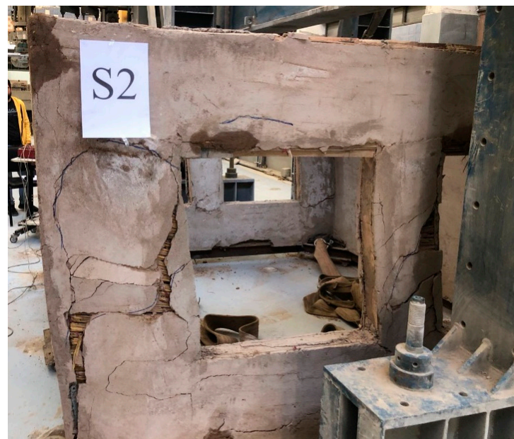
Figure 18. The infilled specimen at the end of the test.
