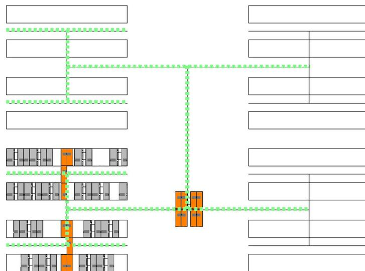
**Figure 6.** Energy grid (energy net green line and orange energy house) and modular units' distribution.
