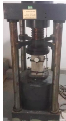
Figure 4. Test setup of elastic modulus of concrete.
