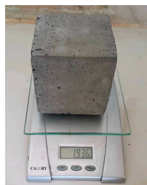
Figure 9. Determination of weight of concrete specimen.
