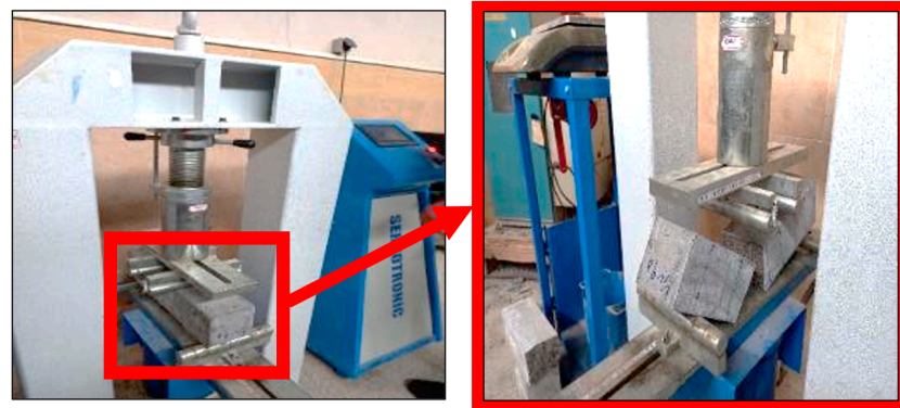
Figure 14. A view of four-point bending test.
