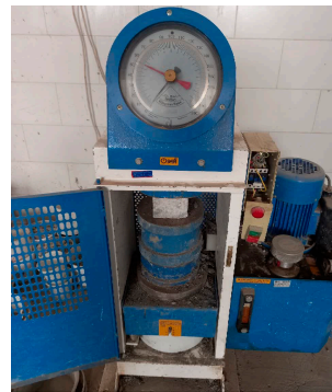
Figure 10. Determination of compressive strength of concrete specimen.
