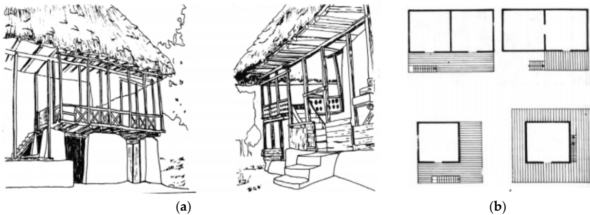
Figure 3. (a) Typical shape of Telar. (b) Different types of Telar in a building plan [14].
