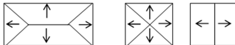
Figure 4. Types of common sloping roofs in the southern margin of the Caspian Sea.
