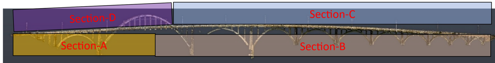
Figure 9. TLS survey phasing plan for Edmund Pettus Bridge.
