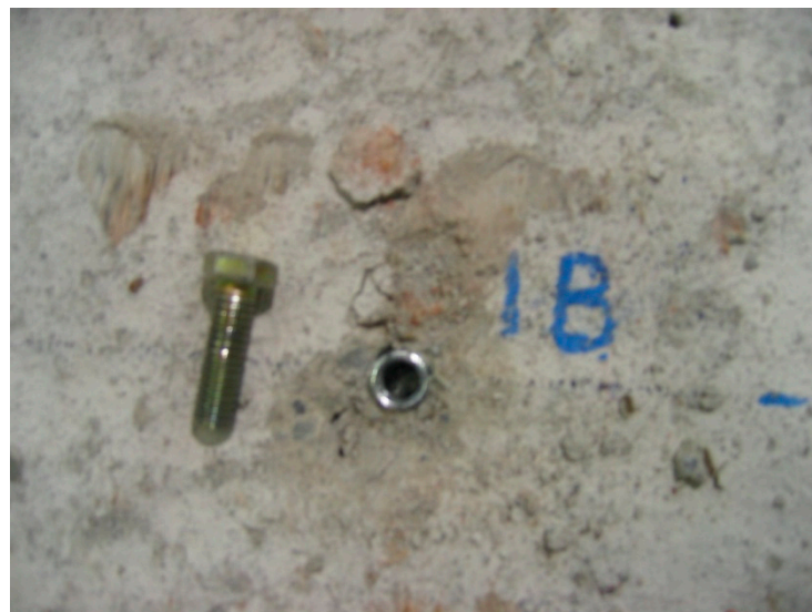
Figure 12. A 9.5 mm anchor after cyclic shear tests at 0.1 and 2 Hz (no shear failure).
