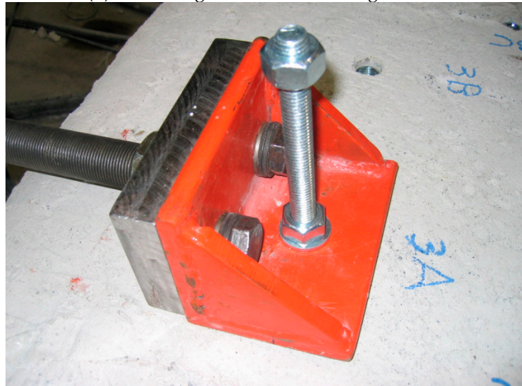
(c) Installed anchor shear connection
