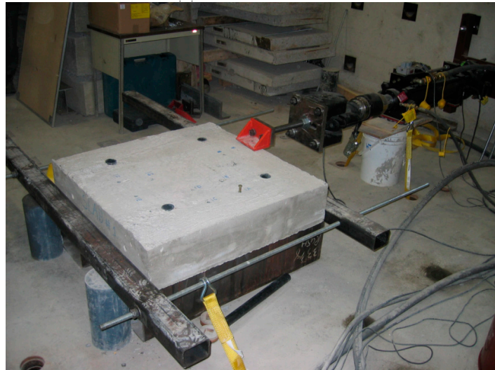
(b) The testing slab before installing anchors
