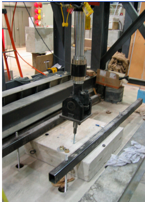
(b) Installed anchor during testing
