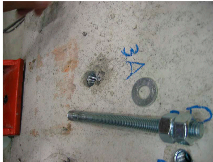
Figure 13. View of the 15.90 mm diameter anchor after a cyclic shear test at 0.1 Hz (no shear failure).
