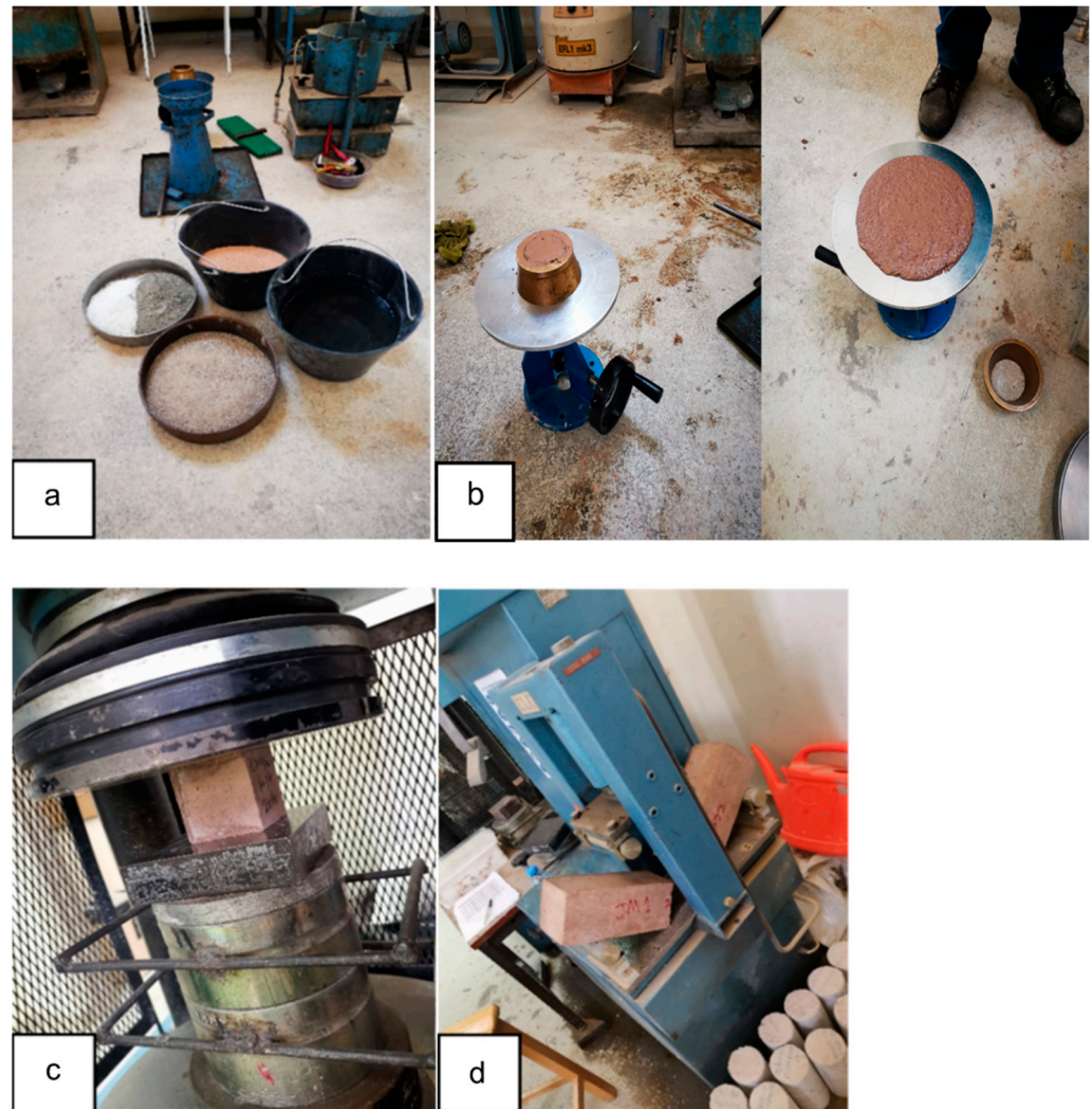
Figure 2. Jointing mortar (a) materials used; (b) flow table test; (c) compression test; (d) flexural test for plaster mortar.
