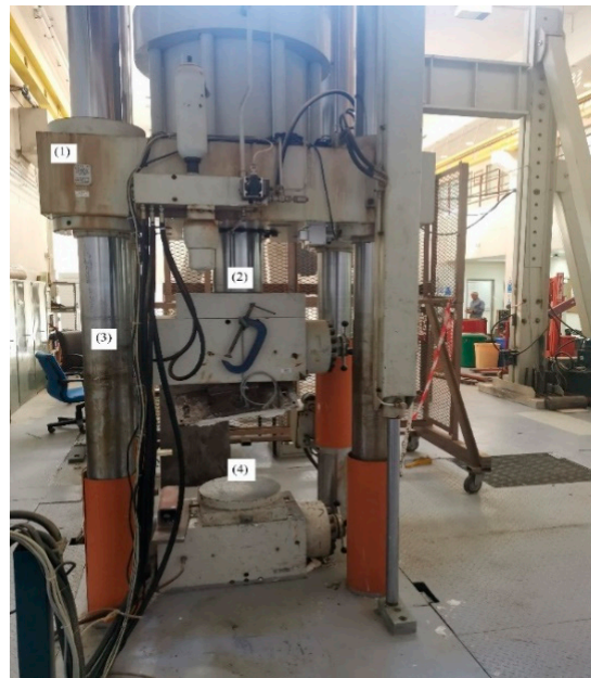
Figure 16. Photograph of Universal Testing Machine: (1) moving crosshead; (2) top actuator loading; (3) load support column; and (4) bottom loading plate.
