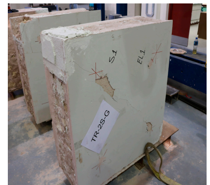
Figure 18. Failure modes and crack patterns. (a) Failure mode of UC wall; (b) Failure mode of TR-1SB wall; (c) Failure mode of TR-2SB wall; (d) Failure mode of TR-2SB-2L wall; (e) Failure mode of TR-2SB-S wall; (f) Failure mode of TR-2SG wall.
