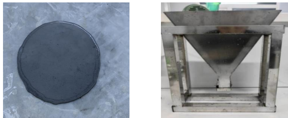
Figure 5. Small slump flow and V-shaped funnel test.
