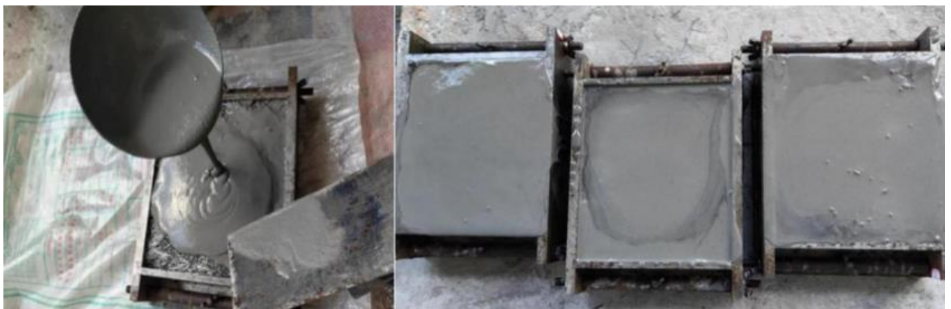
Figure 4. Preparation of SIFCON test blocks.
