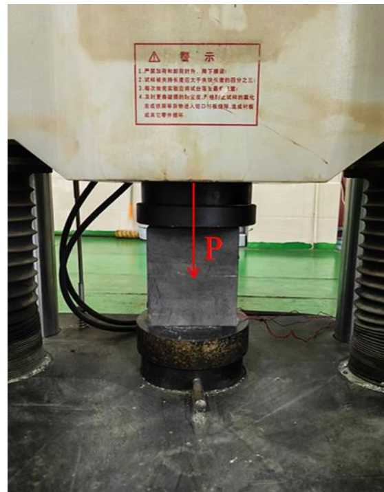
Figure 6. Compression test of SIFCON block.
